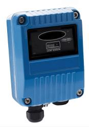
The simultaneous detection of both the UV and the IR light by the sensors will signal an alarm. False alarms from flickering sunlight, arc welding and lighting are eliminated by a combination of UV and dual IR signal processing techniques.
